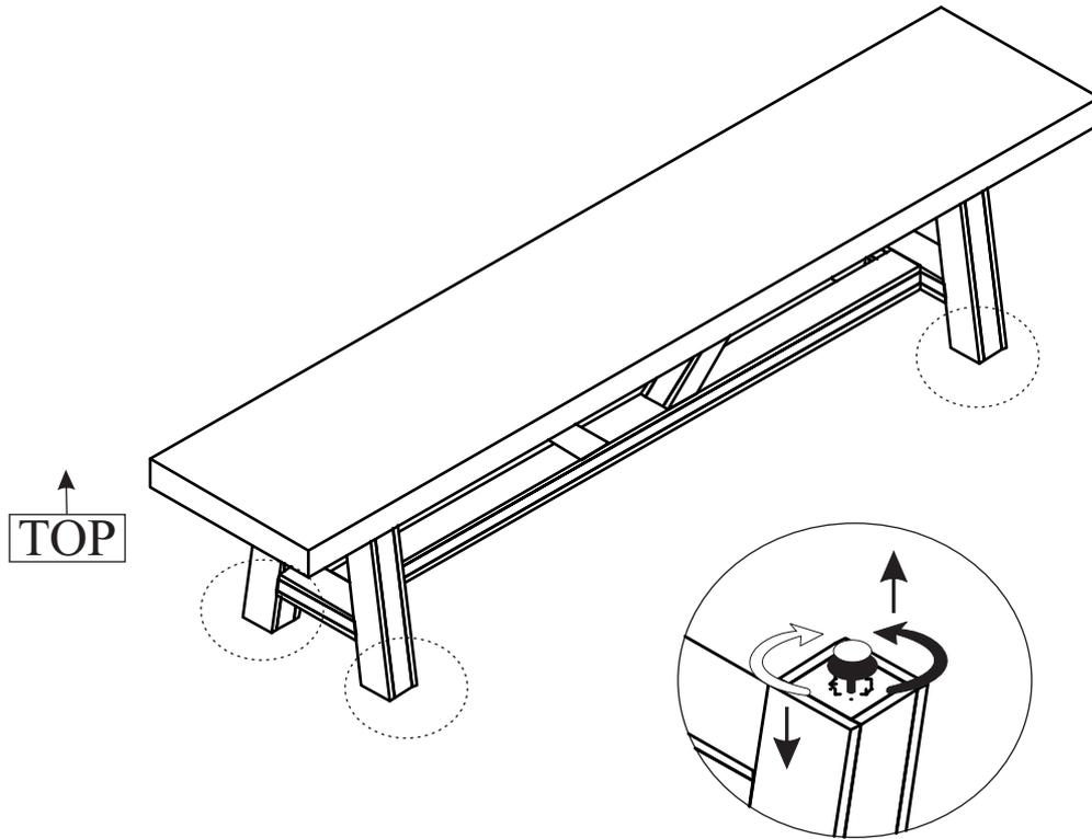
Using a second person to assist you, carefully turn the bench assembly upright. Position the table in its desired location before making any final adjustments using the adjustable floor levelers (if needed). Assembly is now complete and the bench is ready for use.
