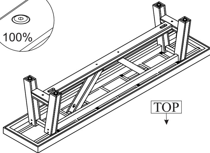
**FULLY TIGHTEN** all Allen Bolts from Steps 1-4 at this time using Allen Key (H-7).
