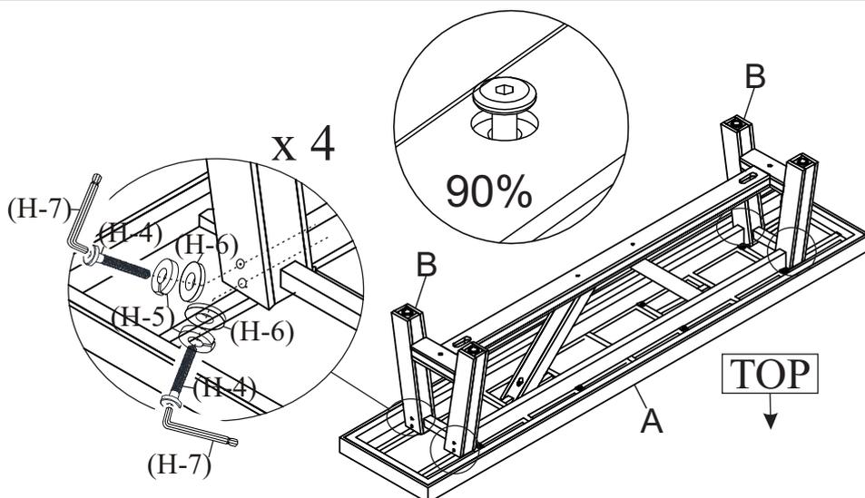
Using a second person to assist you, carefully lower the leg assembly (from Step 2) down onto the Bench Top (A) assembly (from Step 1). Align the holes on Legs (B) with the metal apron frame on Bench Top (A) and secure each leg to the frame using 2 Long Allen Bolts (H-4), Spring Washers (H-5) and Flat Washers (H-6). Engage the bolts using Allen Key (H-7) **but do not fully tighten them yet.**
