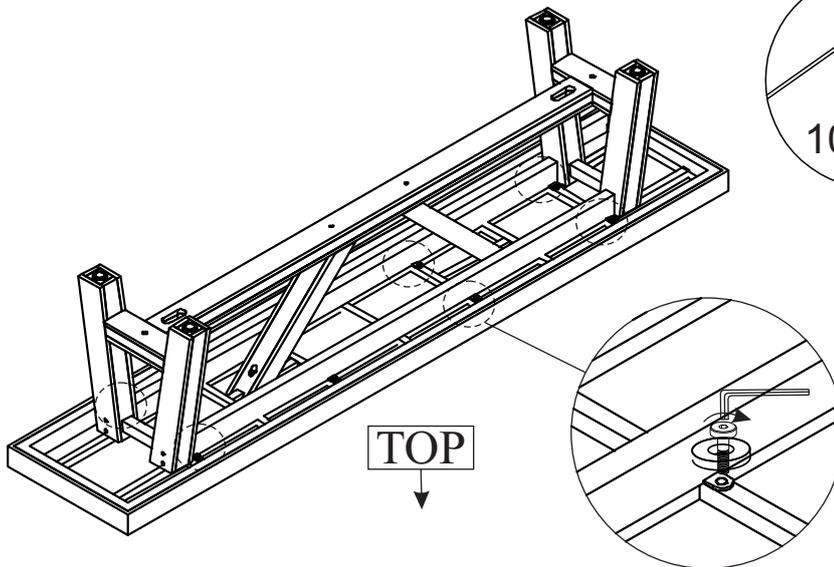
**NOTE:** Bench Top (A) comes with a pre-installed metal frame. Ensure that all pre-installed bolts (12pcs total) securing the metal frame are **FULLY TIGHTENED** using Allen Key (H-7).
