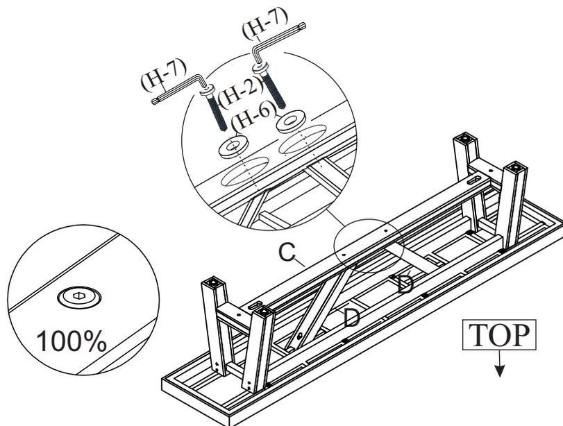
Secure both Upper Wood Support Bars (D) to Lower Wood Crossbar (C) using Medium Allen Bolts (H-2) and Flat Washers (H-6). Engage the bolts and then **FULLY TIGHTEN** them using Allen Key (H-7).
