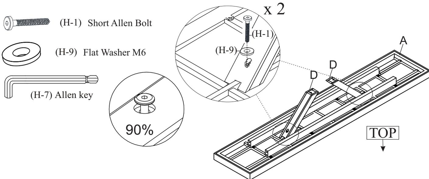
Using a second person to assist you, place Bench Top (A) upside down onto a padded, non-marring surface. Next, position both Upper Wood Support Bars (D) as shown, making sure the notches at the ends of both bars attach over the metal frame on the underside of Bench Top (A). Secure both Upper Wood Support Bars (D) using Short Allen Bolts (H-1) and Flat Washers (H-9). Engage the bolts using Allen Key (H-7) **but do not fully tighten them yet.**
